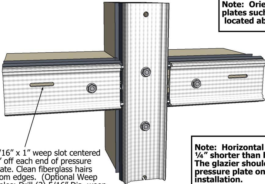
**Note: Orient horizontal pressure plates such that the weeps are located above the mullion tongue**
