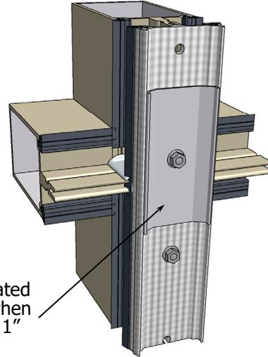
Roll Pin Support located at each horizontal when vertical cover depth 1" and over.
